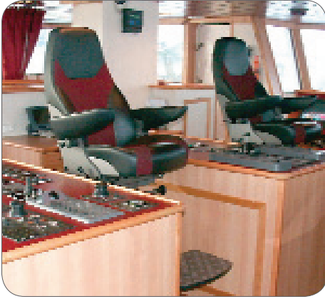
Figure 5: Designed for an offshore oil-drilling rig, this drill-operator control chair was prototyped with an FDM system. Then 25 of its components were manufactured by the same system.
