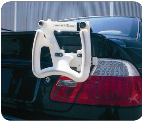
Figure 3. At BMW AG, Regensburg, an FDM system is used to rapid manufacture assembly tools like the one above.
